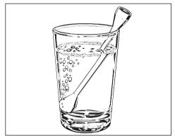
When heating liquids, milk, sauces etc, using microwave power without the boiling rod, the boiling point of the liquid may be reached without the production of typical bubbles. The liquid does not boil evenly throughout. This so-called 'boiling delay' can cause a sudden build-up of bubbles when the container is removed from the microwave oven or shaken, which can lead to the liquid boiling over suddenly and explosively. Danger of injury and damage.
